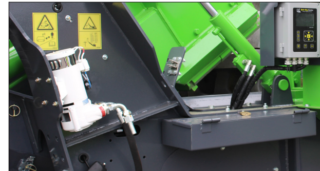
Dust suppression pump
